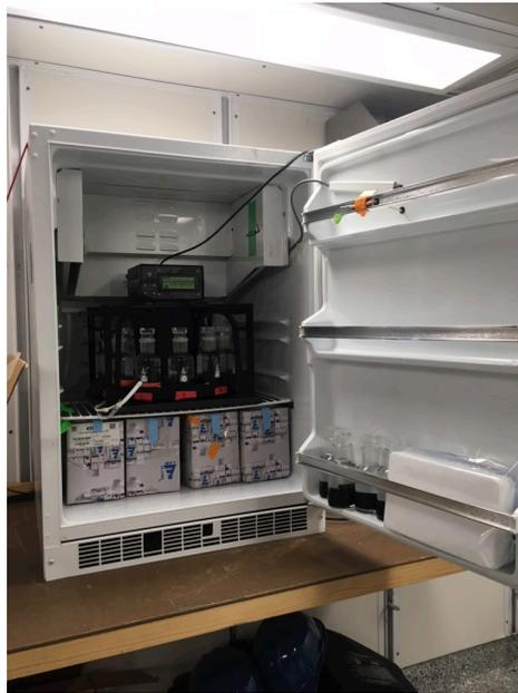
*Figure 12: Photograph of incubator with autoBOD (top shelf) and bottles incubating on the bottom shelf. Extra BOD bottles are in the door of the incubator.*
