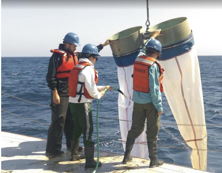
*Figure 9: Photograph from a bongo net recovery.*
