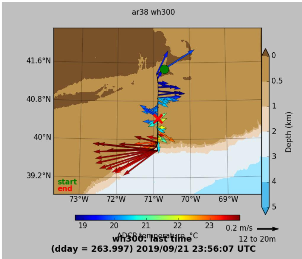
Figure 5: Velocity vectors from the workhorse 300 ADCP
