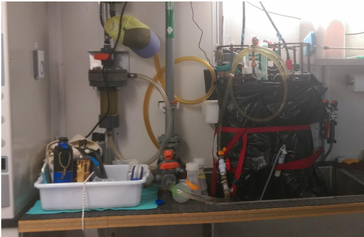
Figure B.8: The underway and discrete IFCB's secured in the forward Main Lab sink.
