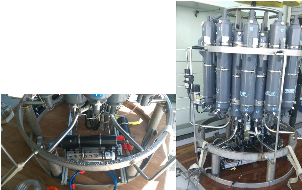
*Figure 13: Final CTD rosette configuration for effective sampling of all instrumentation. Left: The CPICS instrument, associated battery pack, and associated CTD mounted on a T-slot aluminum frame at the past of the Armstrong rosette. Right: The chlorophyll and CDOM fluorometers mounted higher on the frame (left center) on the opposite side of the CTD frame from the CPICS (lower right). The SUNA was mounted on the opposite side of the CTD facing away relative to the CPICS.*
