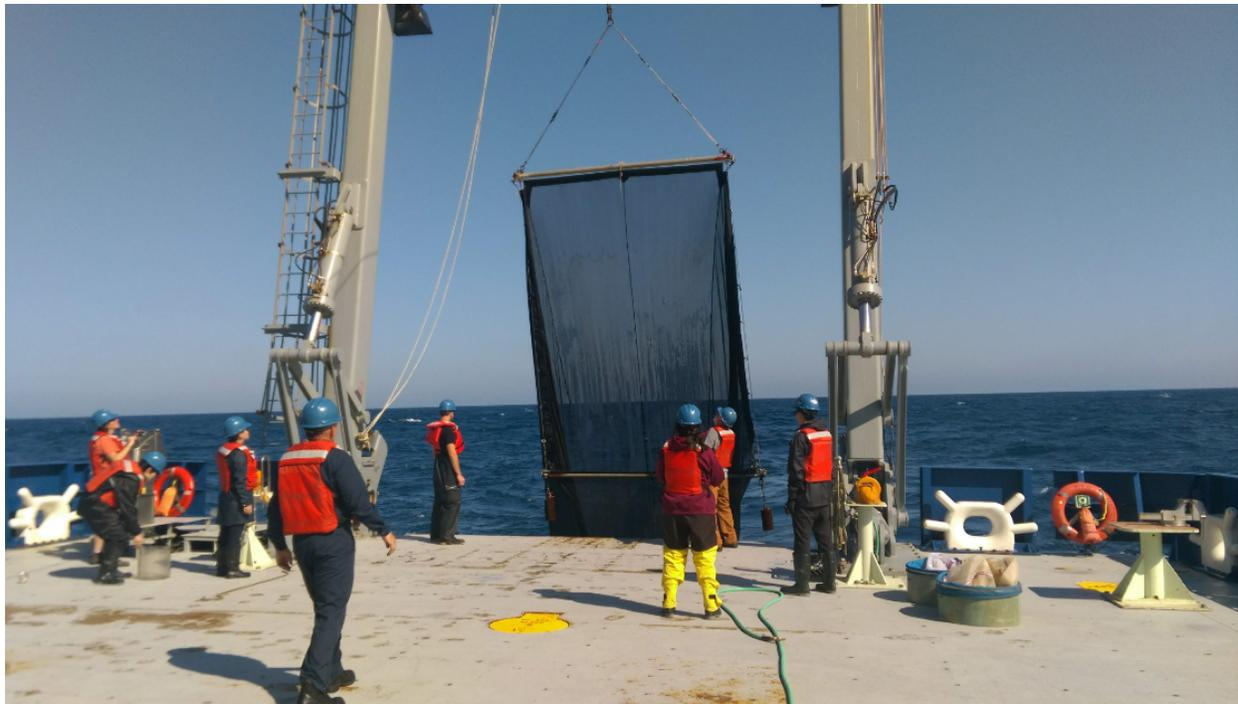
Figure B.1: Midwater tucker trawl being deployed off the stern of the Armstrong.
