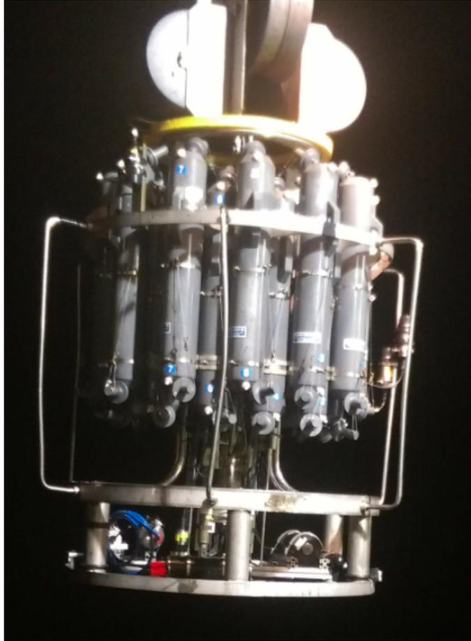
Figure B.9: A 2<sup>nd</sup> view of the CPICS (bottom left), SUNA (bottom right), and fluorometers (right, centered vertically) mounted in a working configuration during a CTD deployment.
