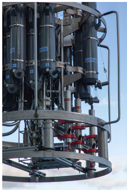
Figure B2: The AR41 shipboard rosette showing stand-alone CTD sensor attachment points
